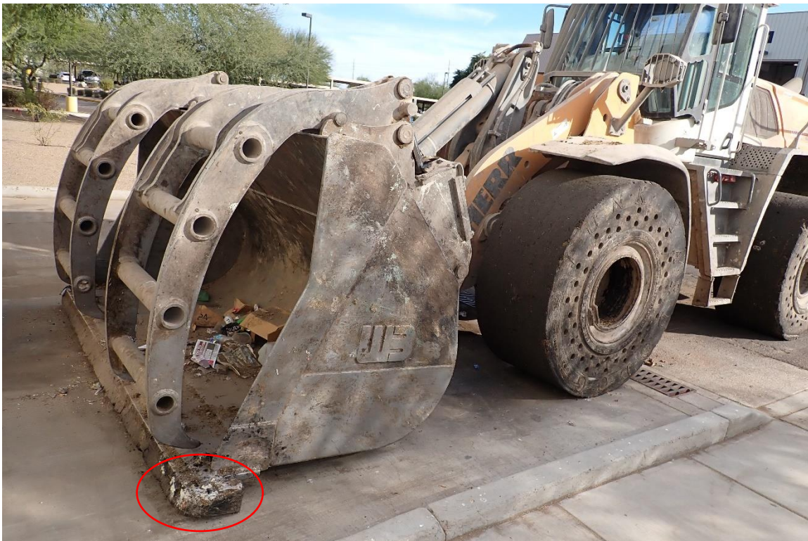
Front end loader with rubber tires and rubber "squeegee" on blade-circled in red
